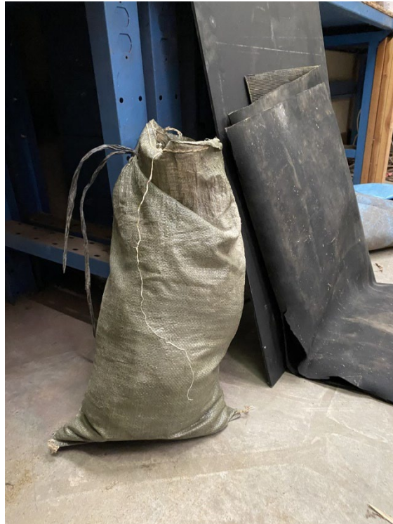
Sandbags used under weirs - ~ 30 – 40 lbs.
