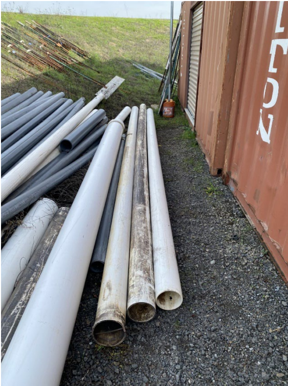
Pipes that go into weirs - 30 – 40 lbs. (2-person lifts)
